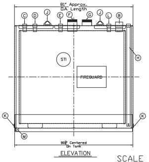
Surface Prep: Brush Blast Paint: Polane White Testing: Per STI Firegaurd Operating Pressure: Atmospheric Estimated Dry Weight: 4,500lbs
